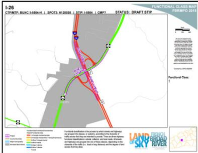
**Functional Classification Map:** shows the different roadways in the project area by functional class. The functional classification helps to define the role of the roadway in accomplishing the many and diverse needs of our transportation system.
